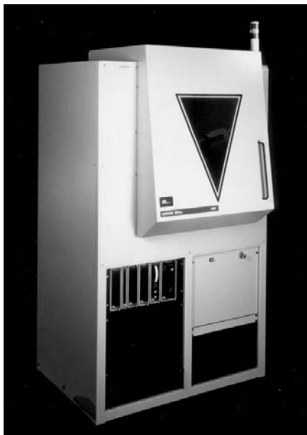
Figure 1 \theta - \theta configuration and exclusive peltier-cooled solid-state detector for optimum performance in X-ray powder diffraction.
